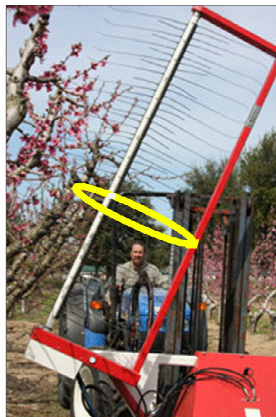
Fig. 9. Mechanical thinner. Prototype for seedling trees would have scaffold push/spacing bar (highlighted in yellow) and brush length reduction to 8 ft.).
