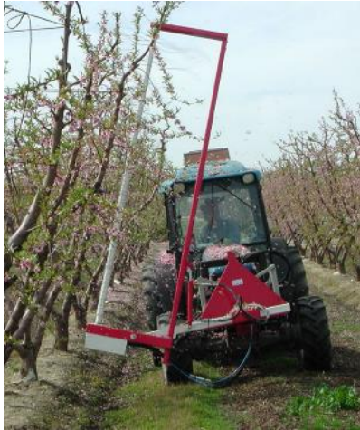
Figure 15. Using the Darwin set up the mechanically thin a peach flowering wall at the UCD evaluation plots.
